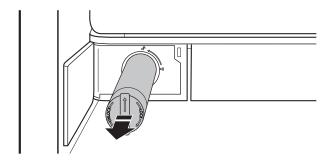
Remove the water filter cap from the water filter being replaced.
