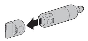
5. Install the water filter cap onto the new filter. Be sure to align the arrows so the groves in filter align with ribs in filter cap.
