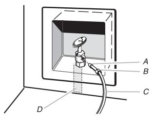
A. Sleeve C. Copper tubing (to refrigerator)
