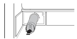
7. Twist the water filter and turn 90° clockwise until it locks into place and the arrows are aligned.
