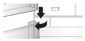
2. Twist the water filter and turn 90° counterclockwise to unlock.
