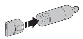
6. Insert the filter into the housing.
